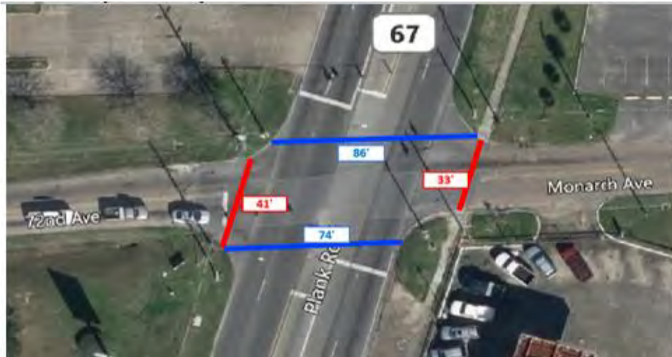
Figure C- 2: LA 67 (Plank Road) at 72nd Avenue / Monarch Avenue Pedestrian Clearance Paths
