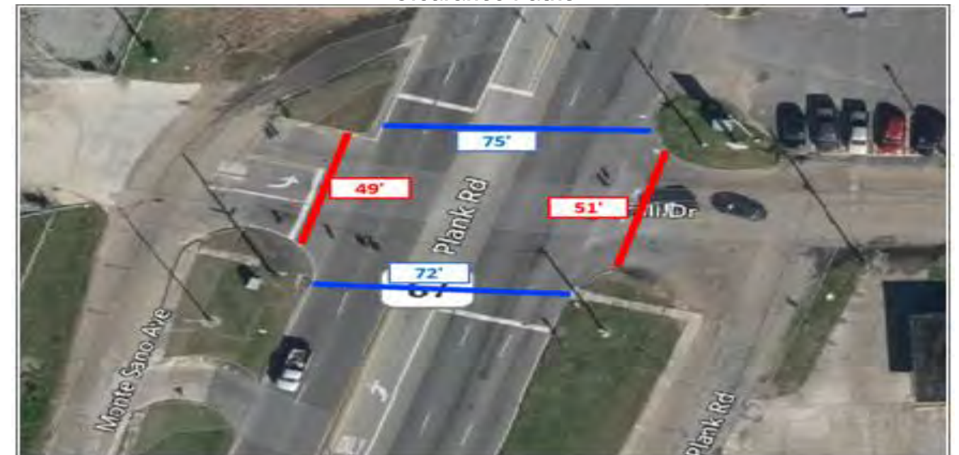
Figure C- 1: LA 67 (Plank Road) at Sumrall Drive / Monte Sano Avenue Pedestrian Clearance Paths
